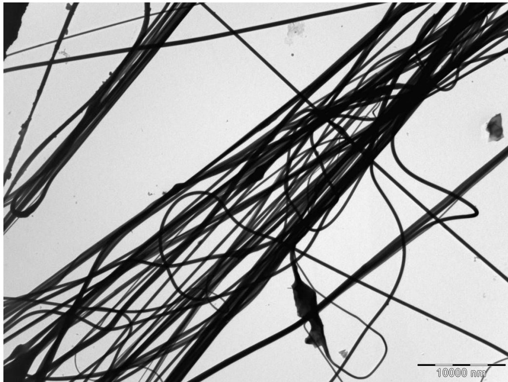
Figure 32: Low magnification HRTEM image of electrospun collagen- 5% SWCNT.
