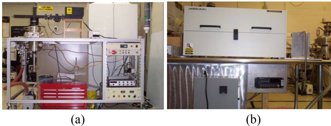
Figure 5: An ASTeX MPCVD system (a), and a one stage furnace CVD system (b) for carbon nanotube growth.
